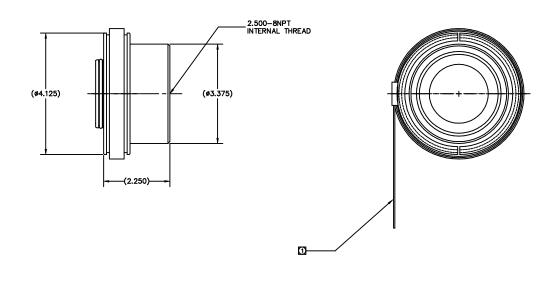
THE HW30-113 HOSE CLAMP IS USED TO ASSEMBLE THE ADAPTER TO THE VR301 NOZZLE.
